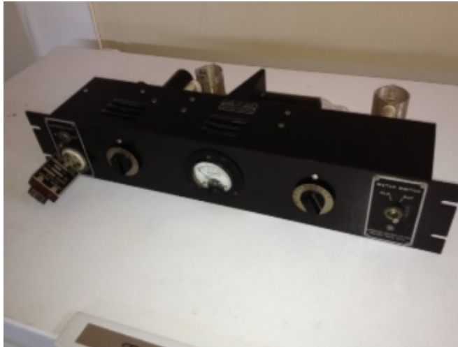
The 1947 Millen 90800 transmitter. 6L6 osc, 807 amp.
