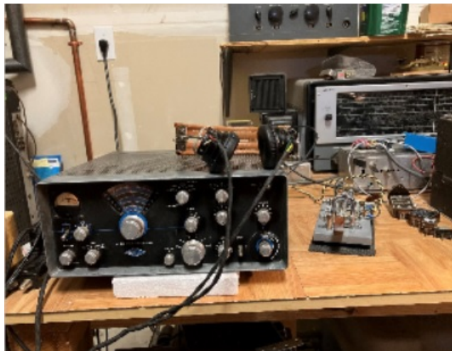
My Dad's Gonset G76 CW/AM transceiver. The only medium power high level plate modulated HF tube transceiver. Pretty broad on CW though.
