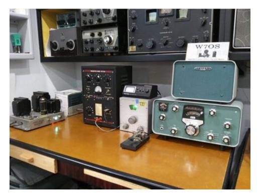
We scrambled to find a VFO that worked well with the Harvey Wells TBS-50A (of course we call him "Harvey") – a couple of HG-10s did not seem to provide enough output, and we went with the VF-1 powered by the low B+ and filament feeds of a Heathkit HP-20 power supply. The first attempt toasted the oscillator tube because the HP-20 provides 12V filaments by default (\$#&\*!). Once the PS was properly jumpered and the tube replaced with a NOS JAN 6AU6, the VF-1 proved rock solid after warm-up.
