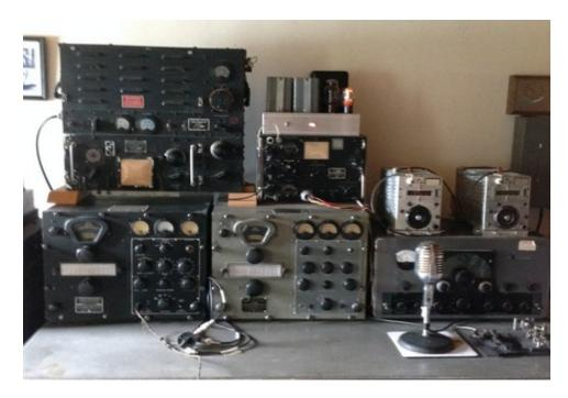
The Navy RBC-1 receiver is the gray receiver on the desk, while the TCS-13 Navy transmitter with HB Power Supply is atop the RBC.
