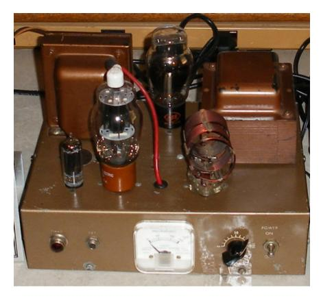
This is a Novice transmitter made in Montgomery AL possibly around 1958. There is still some mystery around this rig since I have no manual, paper work, and I've found nothing on the web, etc. The TN-75 is a 40/80M transmitter using a 6CL6 for the oscillator and an 807 for the PA.
