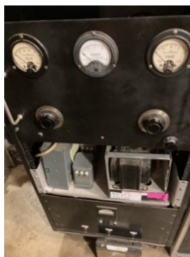
Homebrew 808 based amplifier - 40M (left) 80M (right)
