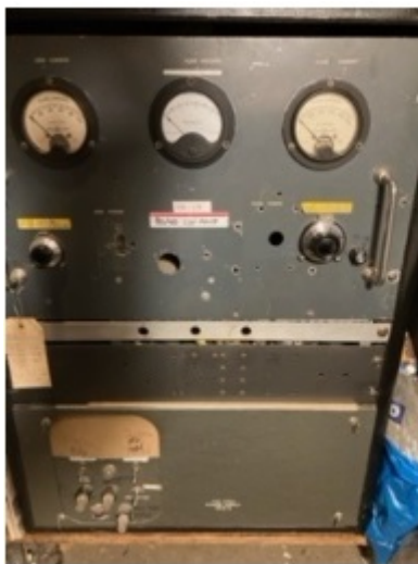
Homebrew 808 based amplifier - 40M (left) 80M (right)
