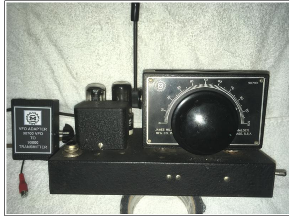
1945 Millen 90700 VFO which runs only on 3.5 Mhz and drives the Millen 90800 transmitter.
