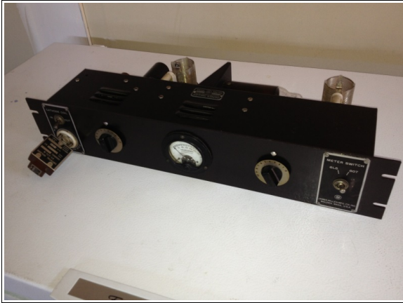
Millen 90800 transmitter (circa 1947, crystal control, 6L6/807, about 25W out)
