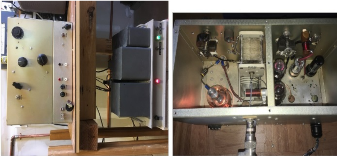
The Henry ISM RF Generator with PS (L) and inside (R) Told you it wasn't pretty!
